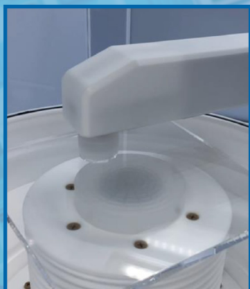
Process Chamber with Point Nozzle Scanning
